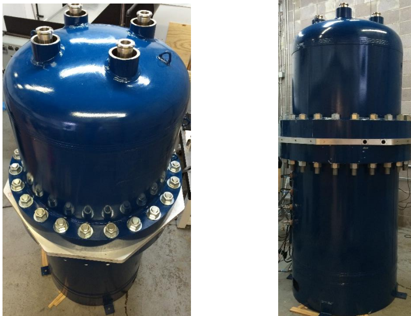
Fig 4) left: 25kW ThermoHeart® Engine. The penetrations in the upper pressure vessel are the thermal heat transfer oil inlets and outlets. The heat rejection fluid is circulated through the center aluminum plate.
