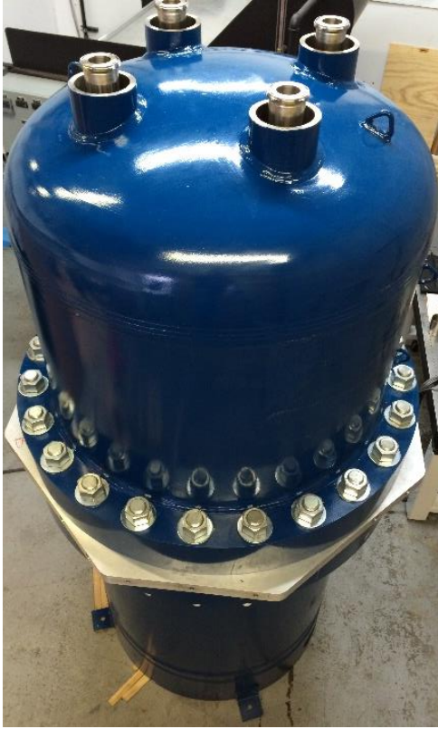
Fig 5) left: 25kW ThermoHeart® Engine. The penetrations in the upper pressure vessel are the thermal heat transfer oil inlets and outlets. The heat rejection fluid is circulated through the center aluminum plate.
