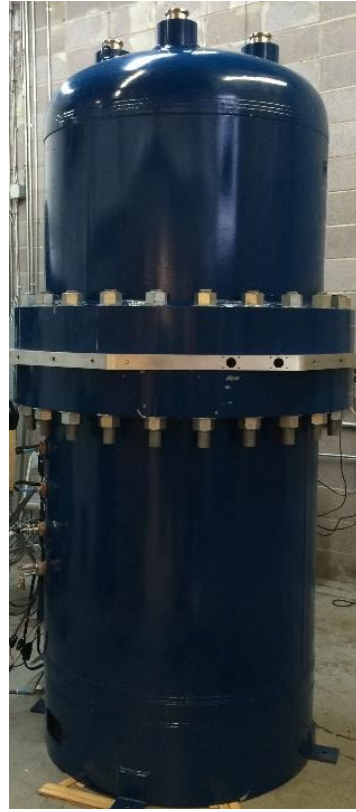
Fig 5) left: 25kW ThermoHeart® Engine. The penetrations in the upper pressure vessel are the thermal heat transfer oil inlets and outlets. The heat rejection fluid is circulated through the center aluminum plate.
